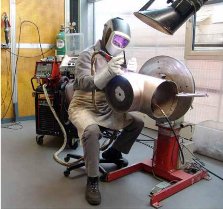
TIG welding 3<sup>rd</sup> weld run in joint with pulled T piece
