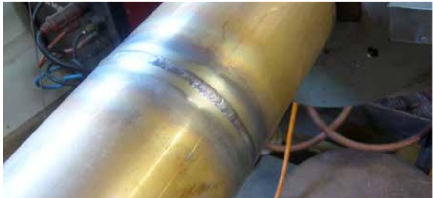
Butt weld showing area which had been cleaned after welding (Courtesy Eucaro Buntmetall GmbH)
