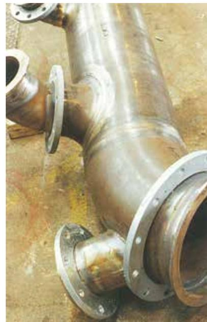
90-10 copper-nickel pipe fabrication for ship seawater system
