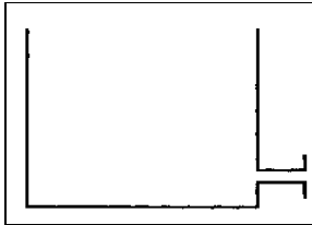
Figure 14-7 Side outlet, above bottom – poor.
