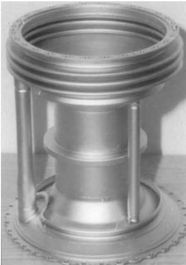
Figure 33 The service life of this flexible bearing support has been extended by electroless nickel plating.
