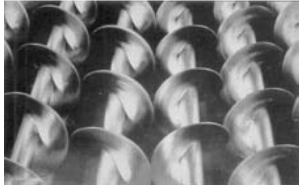
Figure 21 Wear on meat grinding equipment is greatly reduced by electroless nickel.
