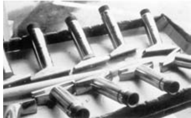
Figure 25 Rams on blowout preventors are plated to prevent corrosion and physical damage.
