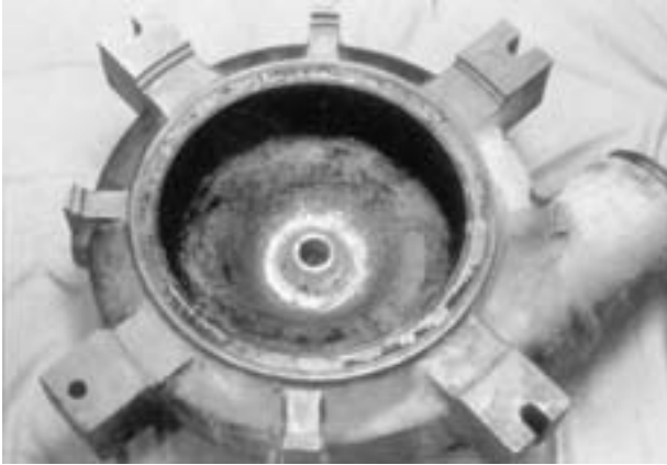
Figure 17 The excessive wear of this aluminum pelletizer for polyethylene was overcome by electroless nickel plating.
