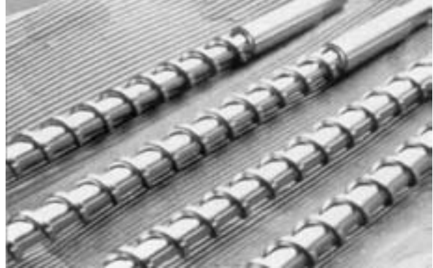
Figure 27 Corrosion and wear of down hole drill motor rotors are resolved by electroless nickel plus chromium plating.
