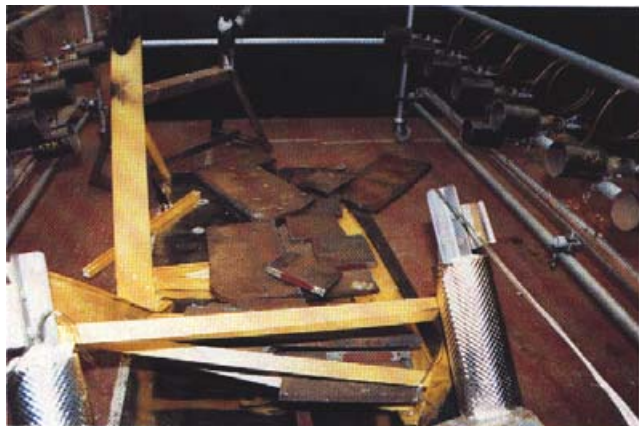
Top left: GRP ladder after fire resistance test. Total collapse occurred before all burners were alight. Smoke and fume emissions were noted.
