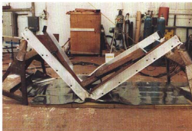
Top right: Aluminium ladder after radiation resistance test. Structural failure occurred after 12 minutes of radiant heating.
