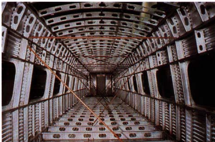
Swedish railcar fabricated entirely from stainless steel (18% Cr 9% Ni). The body has a strong cross-section of arc-welded beams with longitudinal side-beams at floor and ceiling level. Roof and side panels are corrugated and the floor is pattern rolled for further strength.
