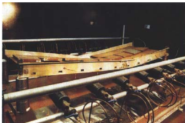
Bottom left: Galvanised mild steel ladder after fire resistance test. Structural integrity was maintained for the stipulated 5 minutes, at which time central deflection was 166.5 mm. Globules of molten zinc were seen falling during test.
