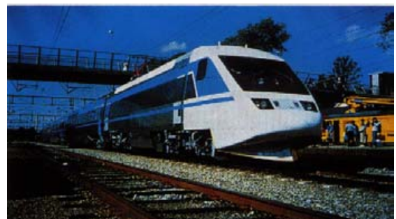
Swedish railcar fabricated entirely from stainless steel (18% Cr 9% Ni). The body has a strong cross-section of arc-welded beams with longitudinal side-beams at floor and ceiling level. Roof and side panels are corrugated and the floor is pattern rolled for further strength.
