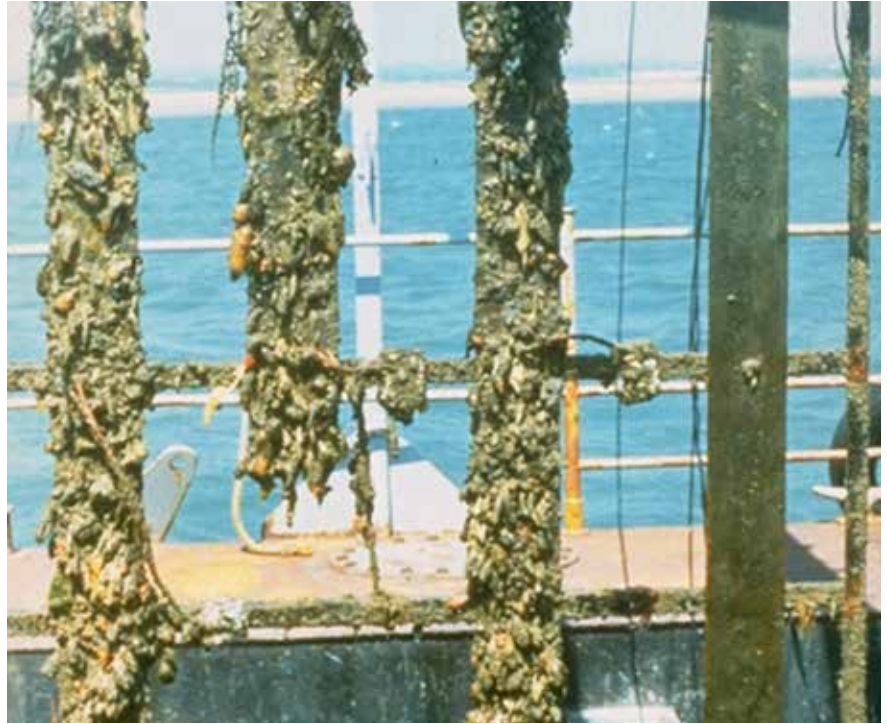
Exposure panels (left to right in above picture): steel, 90-10 copper-nickel sheathed steel, copper-nickel - all three protected with aluminium anodes - and freely exposed copper-nickel. After 12 months exposure at Langstone Harbour, UK, the freely exposed panel remained clean.
