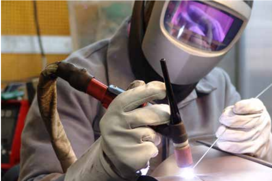
TIG (GTAW) weld process (Courtesy Eucaro Buntmetall GmbH)
