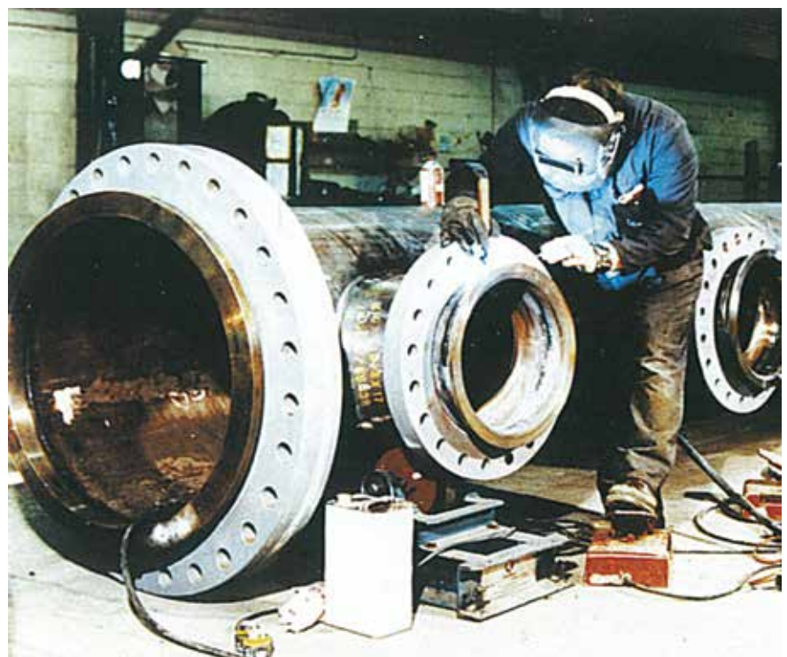
Inlet/outlet manifolds for seawater course filtration unit in 90-10 copper-nickel
