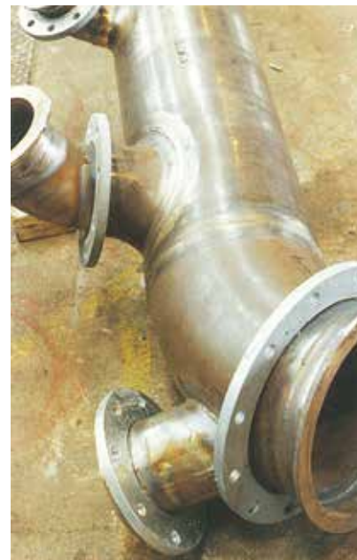
90-10 copper-nickel pipe fabrication for ship seawater system
