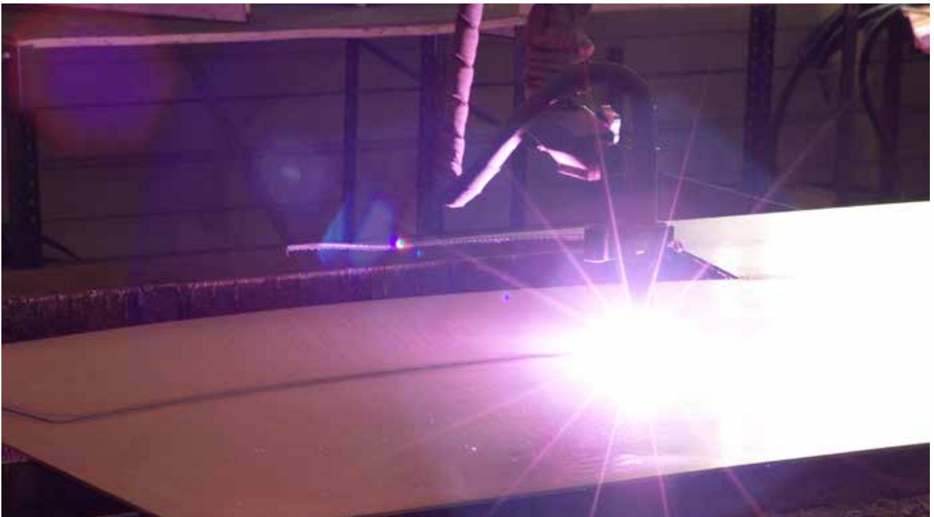
Plasma cutting copper-nickel plate (Courtesy Eucaro Buntmetall GmbH)
