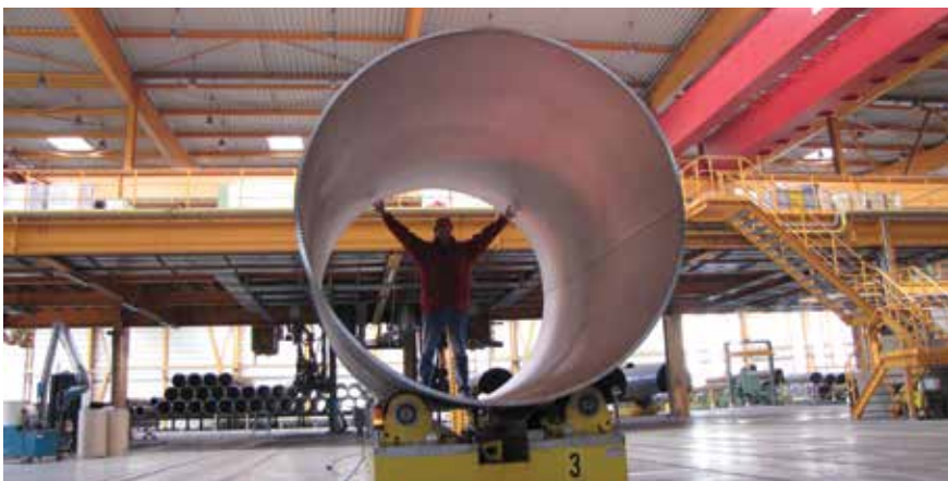
Large diameter steel pipe manufactured with 90-10 copper-nickel inner liner (Courtesy of KME Germany GmbH & Co. KG/Bergrohr GmbH)
