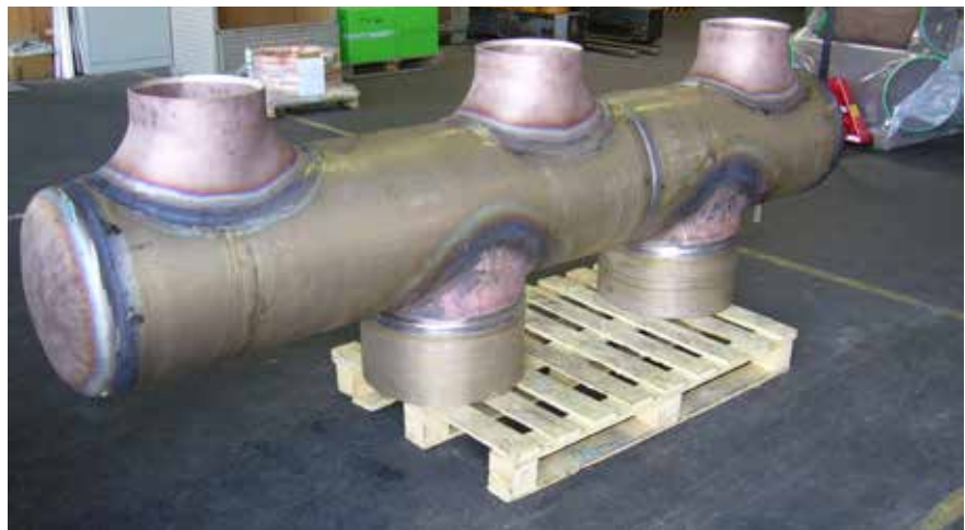
Pipe assembly showing both cold pulled T pieces and welded saddle connections (Courtesy Eucaro Buntmetall GmbH)
