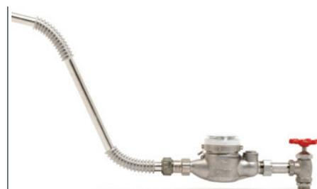
*Tokyo has led the way in successfully using stainless steel partially corrugated tube (SPCT) in water service systems. Since the 1980s, the Tokyo water authority has replaced ageing water distribution systems with stainless steel piping, resulting in high water quality and a significant reduction of water leakage.*
