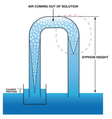
Figure 4 - Diagram showing syphonic air release
