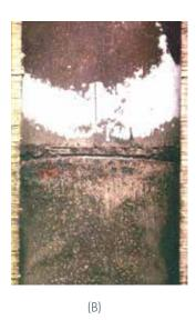
Figure 7 - Ammonia induced attack of 90/10 copper-nickel heat exchanger tube
