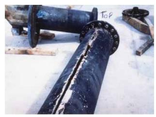
Figure 10 - Corrosion of nickel aluminium bronze pipe along seam weld due to residual beta-phase
