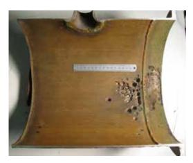
Figure 6 - Pitting attack of 90/10 copper-nickel due to sulphide in the seawater (Courtesy of Intertek)
