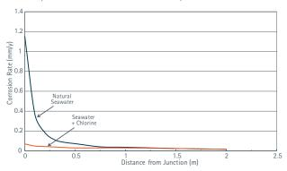
Figure 9 - Effect of chlorine on the corrosion of a 90/10 copper-nickel pipe coupled to one of 6% Mo austenitic stainless steel
