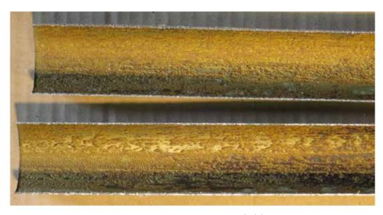
Figure 5 - Severe erosion corrosion of 25.4 mm OD 66/30/2/2 Cu-Ni-Fe-Mn in a dump condenser due to syphonic air release
